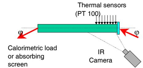
Figure 3: Experimental set-up to observe the heating of the side wall of the waveguide with an IR camera.
