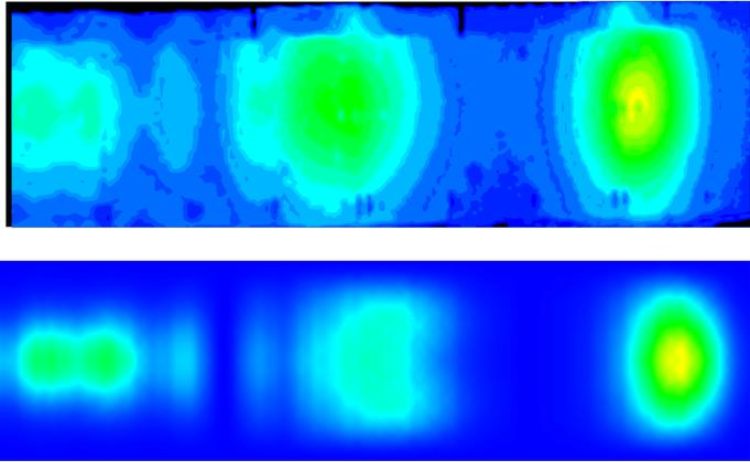
Figure 4: Measured temperature distribution at the outer surface of the waveguide (top) and calculated power distribution at the inner surface (bottom).
