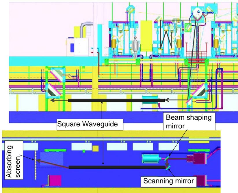
Figure 2: Installations and beam path from gyrotron to square waveguide. The power is transmitted in a quasi-optical line, including polarisers which allow any linear and circular polarisation. The beam power is absorbed in a calorimetric load at the end of the waveguide (not shown here) or on an absorbing screen.
