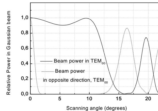
Figure 1: Efficiency of the  $TEM_{00}$  beam in nominal and opposite direction vs scanning angle. Note that power in higher-order modes in this calculation is considered as loss (from [4]).
