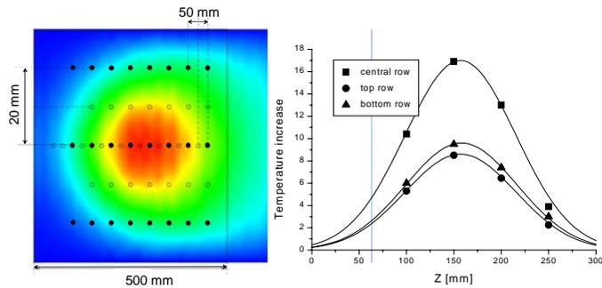
Figure 5: Position of thermal sensors (left) and measured temperature distribution at the end of a 5 s shot.
