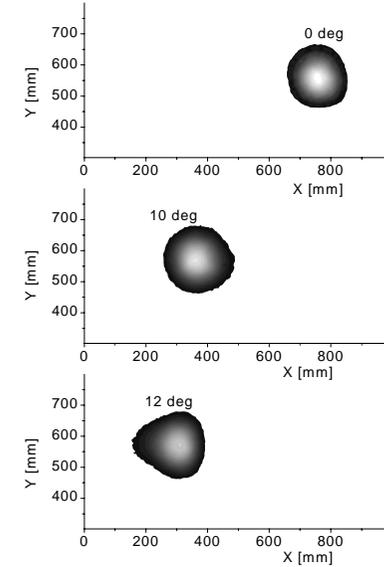
Figure 6: Far field pattern at a scanning angle of  $0^\circ$ ,  $10^\circ$  and  $12^\circ$ . Shown is the temperature increase at the target in a linear scale ( $\Delta T_{\text{Max}} \approx 11$  °C).
