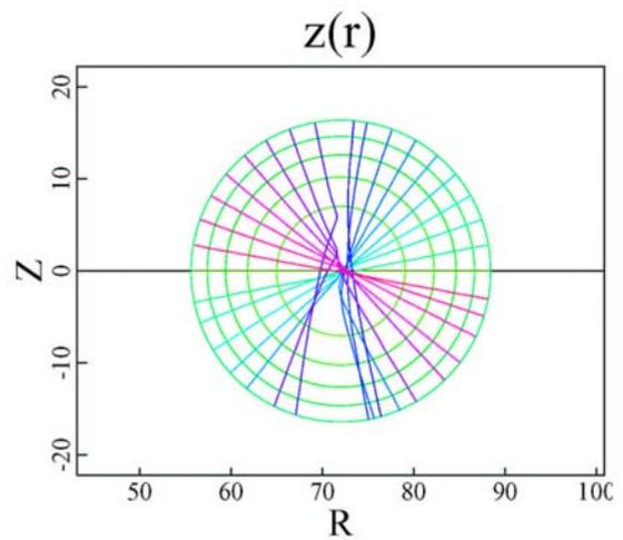
Fig. 2 X-mode second harmonics in RTR for non-Hermitian relativistic dielectric tensor using the dispersion function  $D = \text{Re } \lambda$
