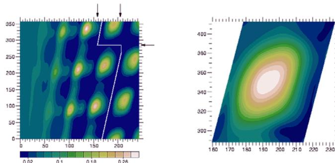
Fig. 2: Power distribution on the launcher wall
