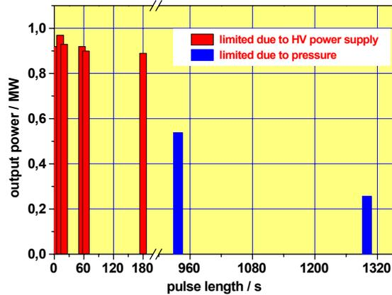
Fig. 4: Output power for different pulse lengths
