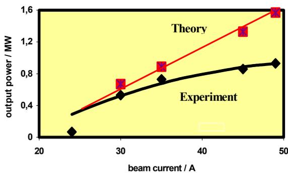
Fig. 5: Output power as function of beam current
