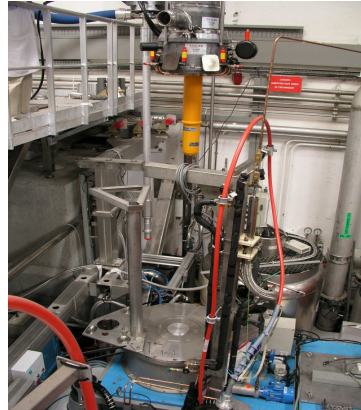
Figure 10. New gyrotron being installed on the test bed
